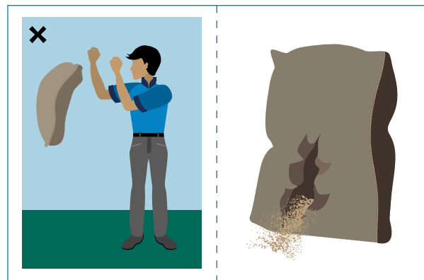
Figure 22: Do not throw or drop this will split any package, especially paper sacks.
