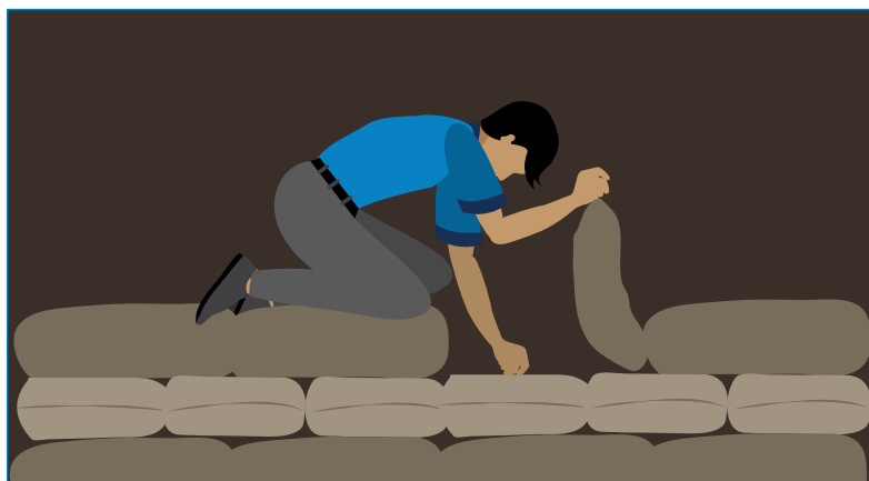
Figure 57: Check for heating, by lifting a top bag and feeling the bag below.
