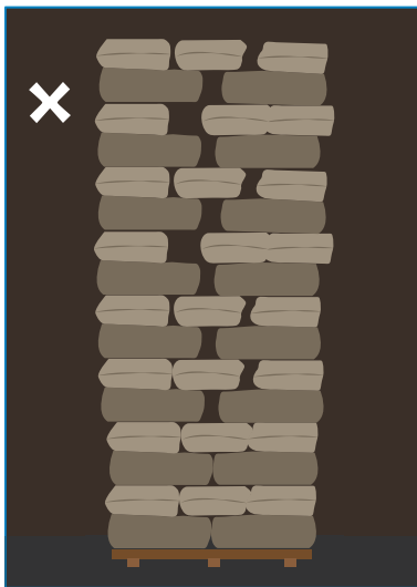
Figure 45: The stack should not be so high that it is unstable.
