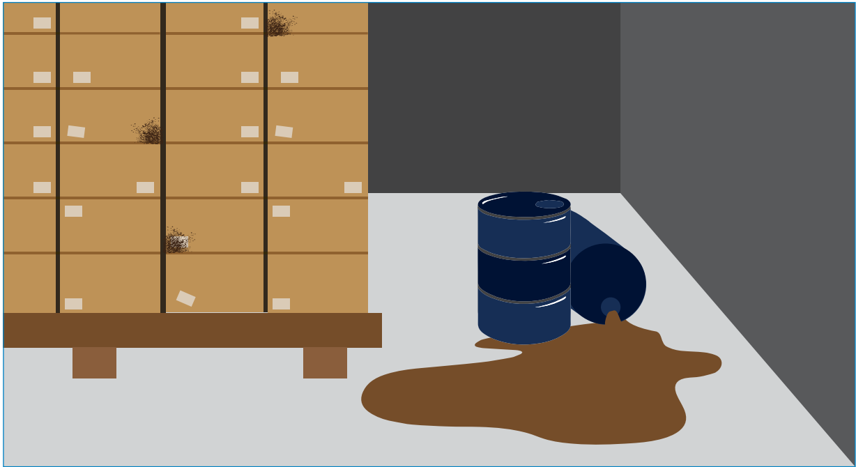
Figure 61: With vegetable oil, look for leaking containers.
