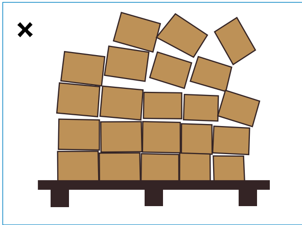
Figure 32: Dunnage should be level, otherwise the stack may be unsafe.
