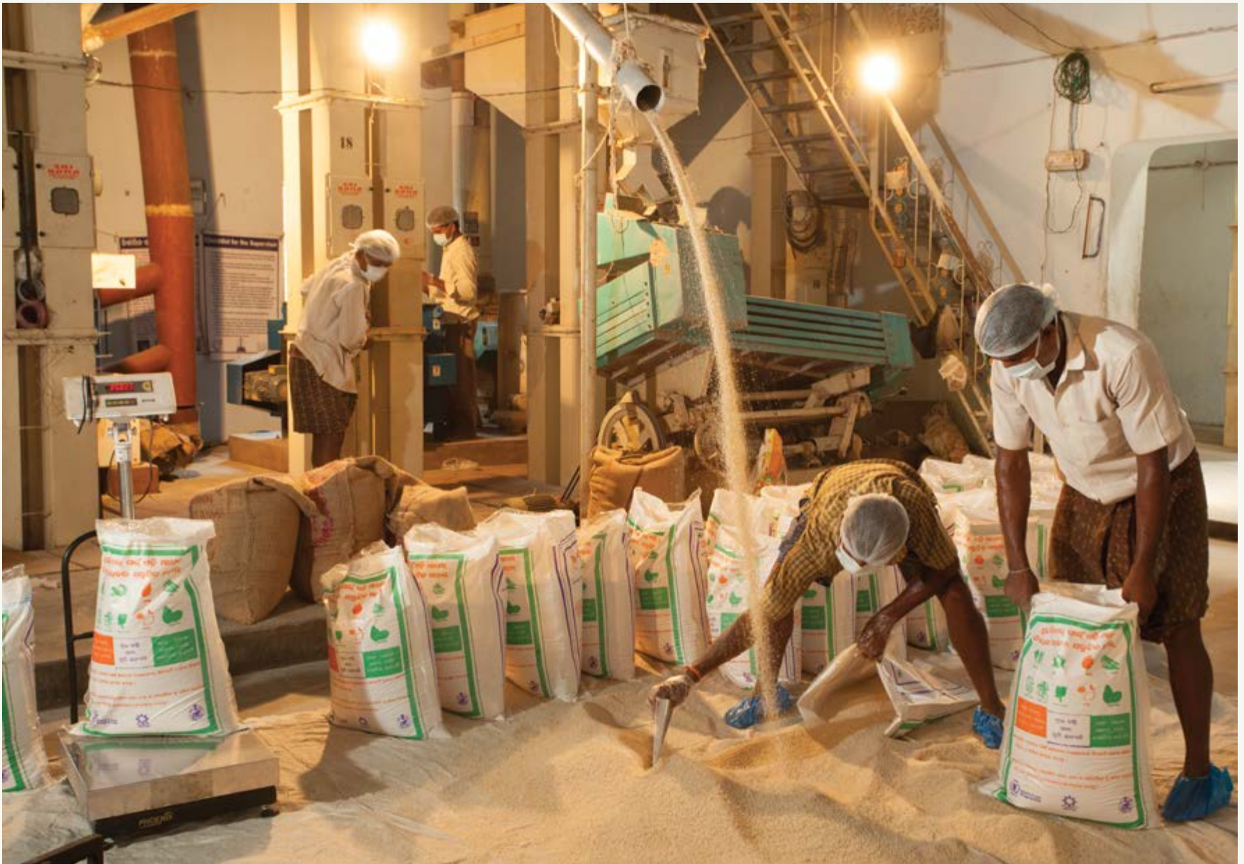
2014, Odisha: Rice mill in Odisha, where fortified rice kernels are blended with regular rice in a ratio of 1:100. This fortified rice is then sent to schools, where it is cooked under the Government's Mid-Day Meal programme and served to children aged six to 14 years.
