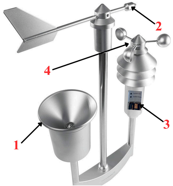
Fig. 5. Parts of the weather station used in the DocuCam Module. Where 1: Rainfall drop collector, 2: Anemometer, 3: Batteries, 4: Sensors (Temperature, Humidity, and Sunshine duration).
